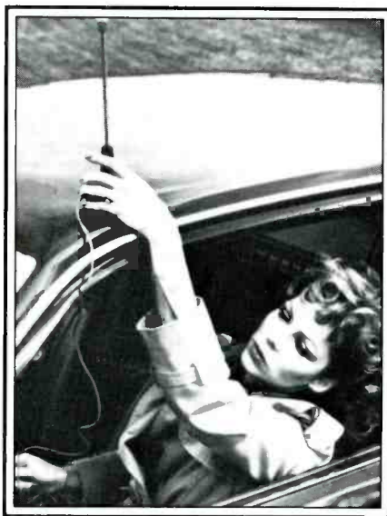
The small 27 MHz AM transceivers use a base loaded magnetic mounted antenna. Some units are designed with telescoping metal whips while others use "rubber duck" types. (Photo courtesy G.E.)
