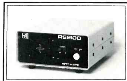
This is the HAL RS2100 RTTY Tuning Scope that shows an accurate display of a received signal.
