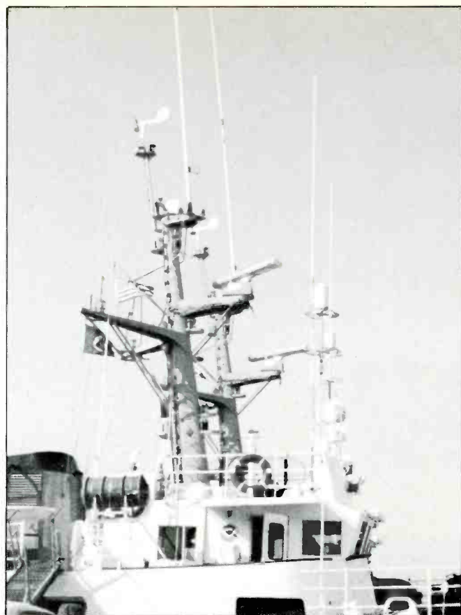
Superstructure of the HECK shows lots of antennas for communicating over a wide range of frequencies. The dual mast shown is misleading since the ship has only a single mast. One of them seen in the photo actually is located atop another NOAA vessel docked on the far side of the HECK.
